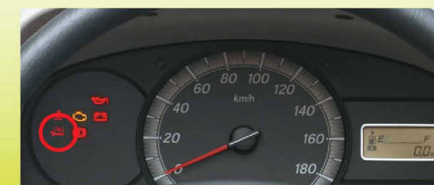
CNG Malfunction Indicator Lamp
